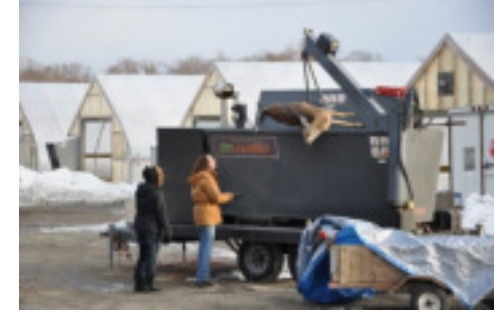
The unit tips hydraulically via remote control to accommodate any loading method.
