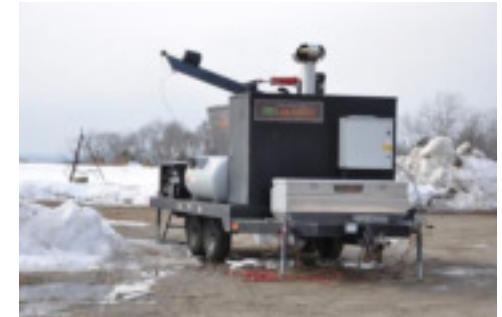
The unit tips hydraulically via remote control to accommodate any loading method.
