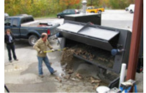
Units tip hydraulically for simple and FAST cycle turnaround. The final bone remains are sterile. Unit is easy to decon before transport away from the disease site.
